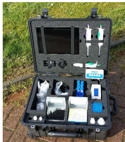
Figure 2 – 2 nd Generation ATP Field Equipment
